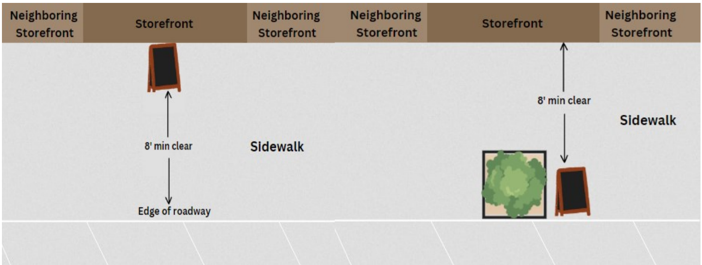
Figure 7—Permitted A-Frame Storefront
